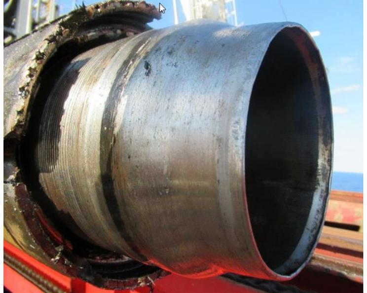
The optimized geometry and toughness of the Glyphaloy cutters allowed the customer to perform the operation in a single trip compared to the competitor's five runs.
