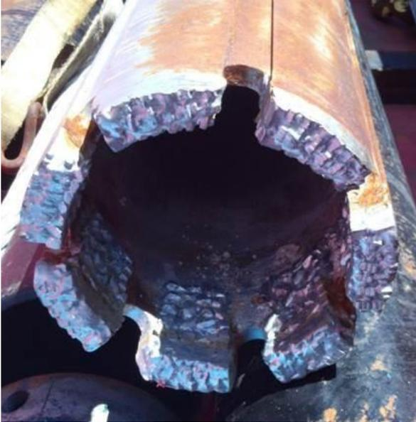
This AMT crown shoe, shown before deployment, incorporates several layers of Glyphaloy carbide cutting structures, which are among the toughest in the industry.
