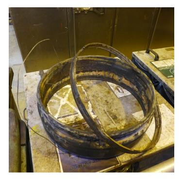
A modified version of the BHGE MASTODON hydraulic pulling tool freed this shallow fish in a matter of mere minutes without any impact on surface equipment.
